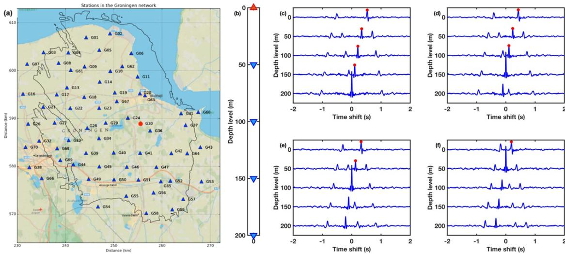
**Figure 1** (a) Map of the borehole stations of the Groningen network. The red filled circle is the borehole we used in our study, G30. (b) Accelerometer (red triangle) and geophones (blue inverted triangle) borehole set up in Groningen. (c-f) Stacks of transverse component cross correlations for virtual sources at different depth levels. The red dots are the travel time picks of upgoing direct S wave that we used in our transdimensional tomography.
